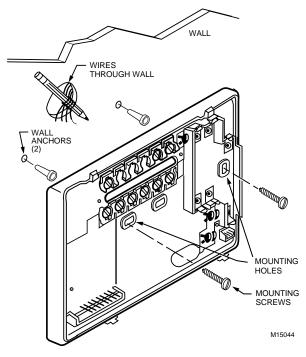
Fig. 2. Mounting the wallplate.
