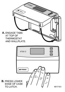
Fig. 5. Mounting thermostat on wallplate.
