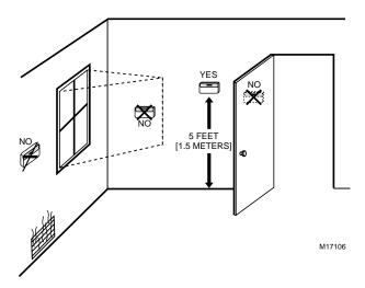
Fig. 1. Typical location of thermostat.
